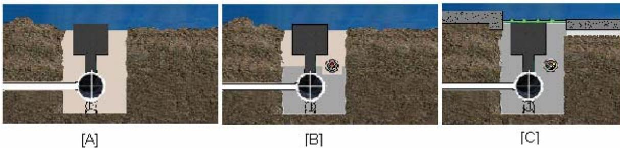
This allows the use of a flowable fill to minimize the excavation required for the pipeline. And the use of elaborate sheeting and shoring [top inset photo] is not necessary because workmen do not have to enter the trench to compact the bedding material in lifts. Polyethylene plastic pipe has the economic advantage over conventional clay, concrete or metal pipe placement.
