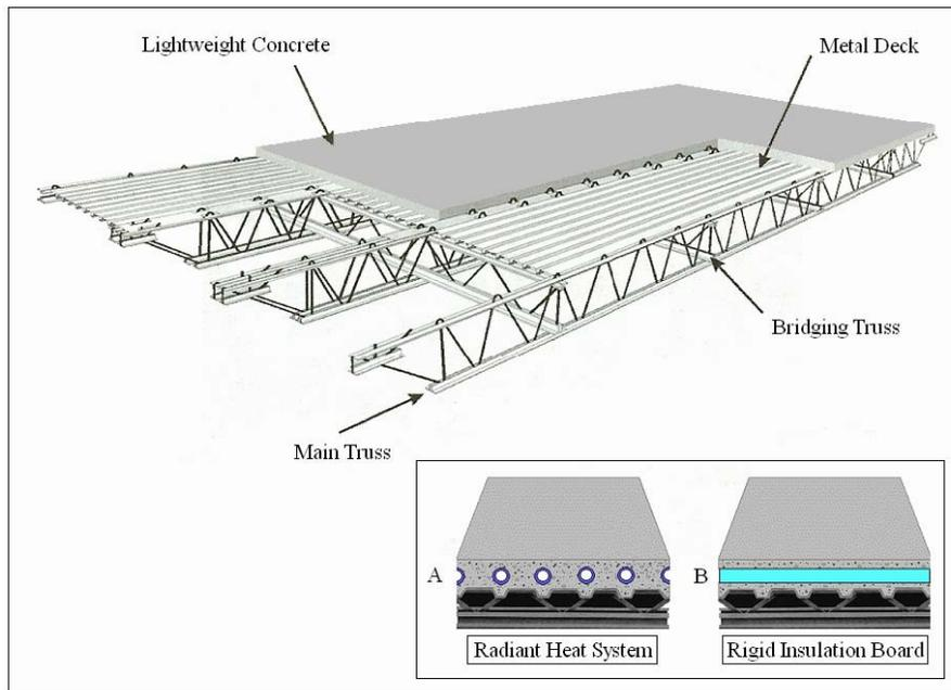
Application for insulated properties as well as a sound barrier for lightweight composite roof or floor deck in commercial, industrial, residential buildings/structures. This would especially true for power utility problems currently being experienced in hot and cold regions where electricity, gas or oil consumption is an issue. Heating and cooling costs are reduced.
